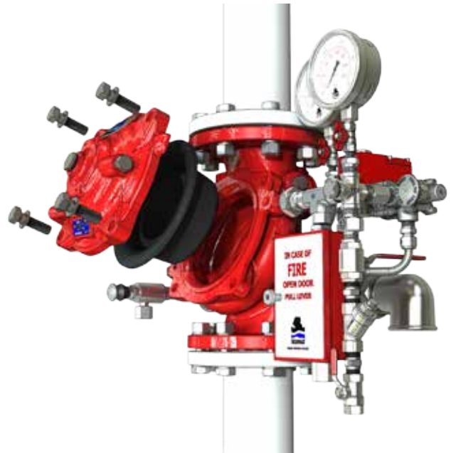
Fig 7: Diaphragm inspection inline and without trim removal
